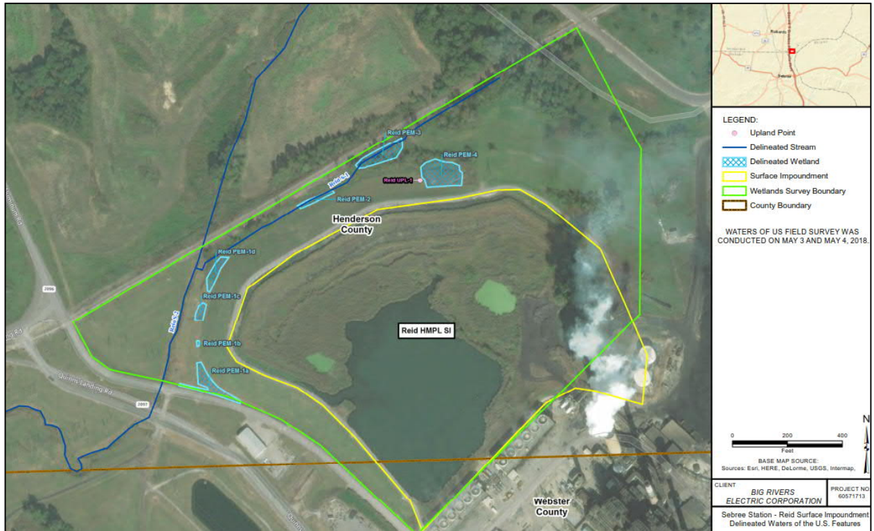
Figure 3: Environmental Features Existing CCR Surface Impoundment
